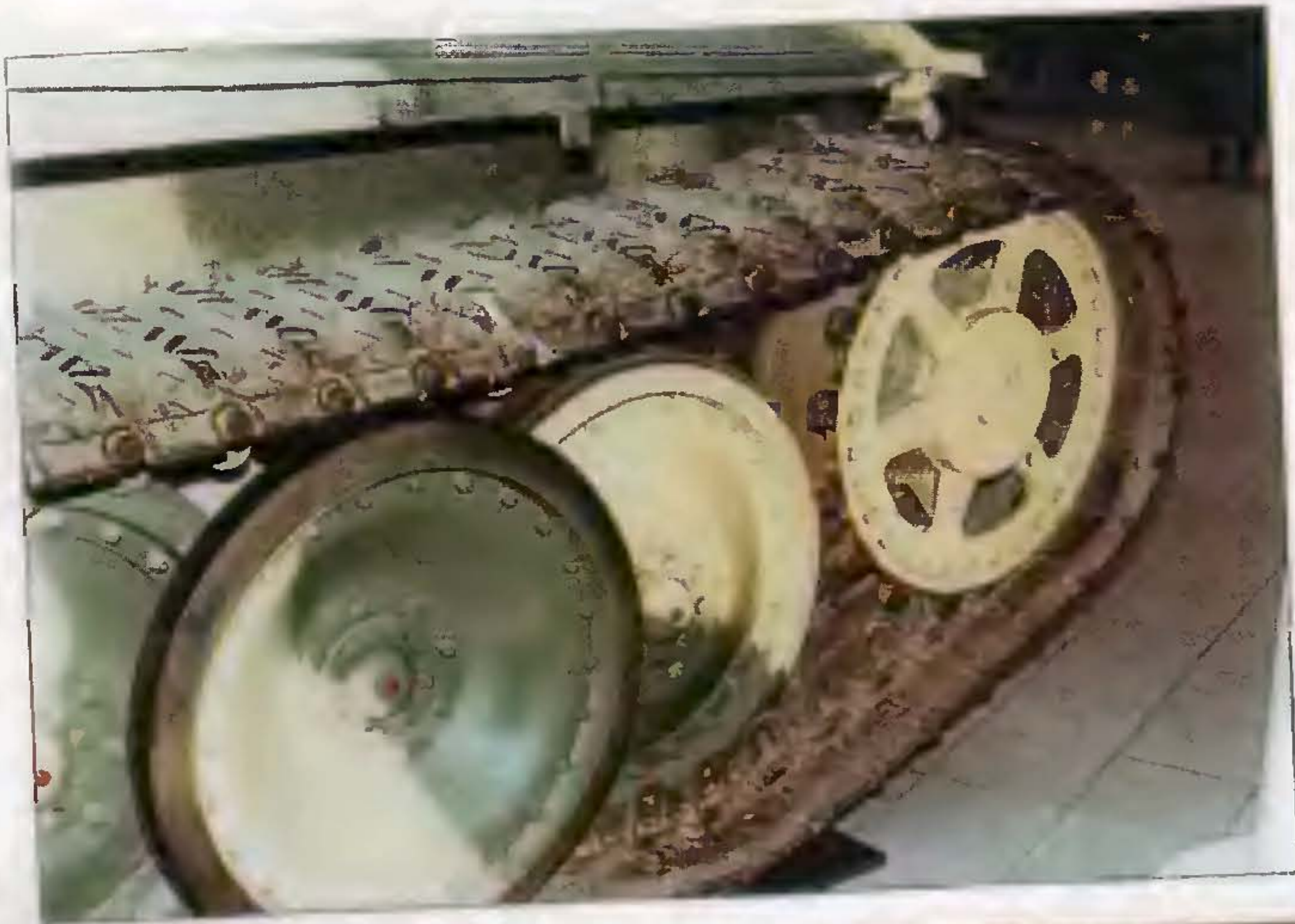
Left. Drive sprocket, road wheels. Below. Road wheels and Kgs 64/660/160 track links with six chevroned cleats.
