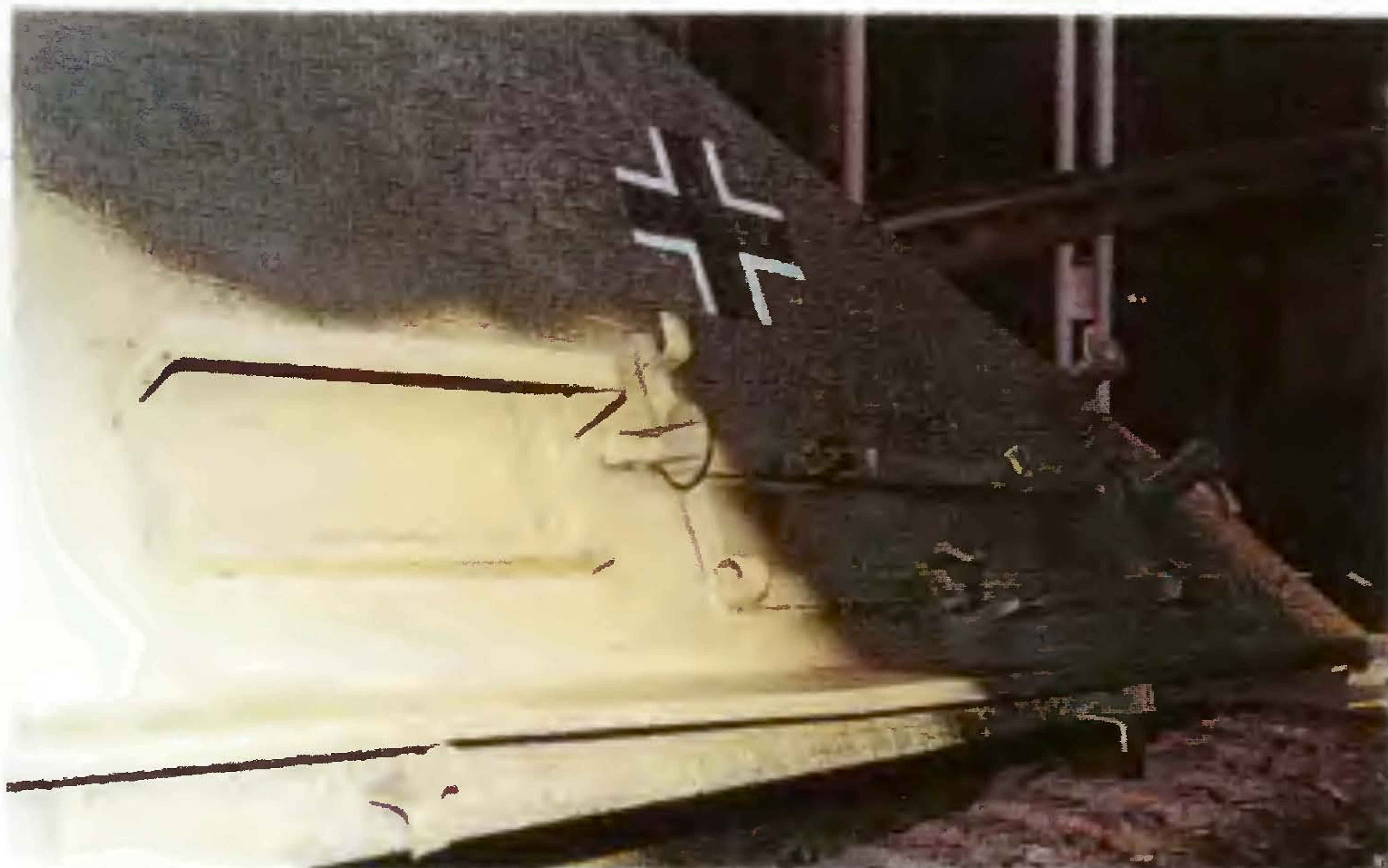
Above. A view of rear armour of superstructure and engine deck. Note on the right a small spent case discharge hatch and above hatch a FuG 5 radio set aerial mount.
