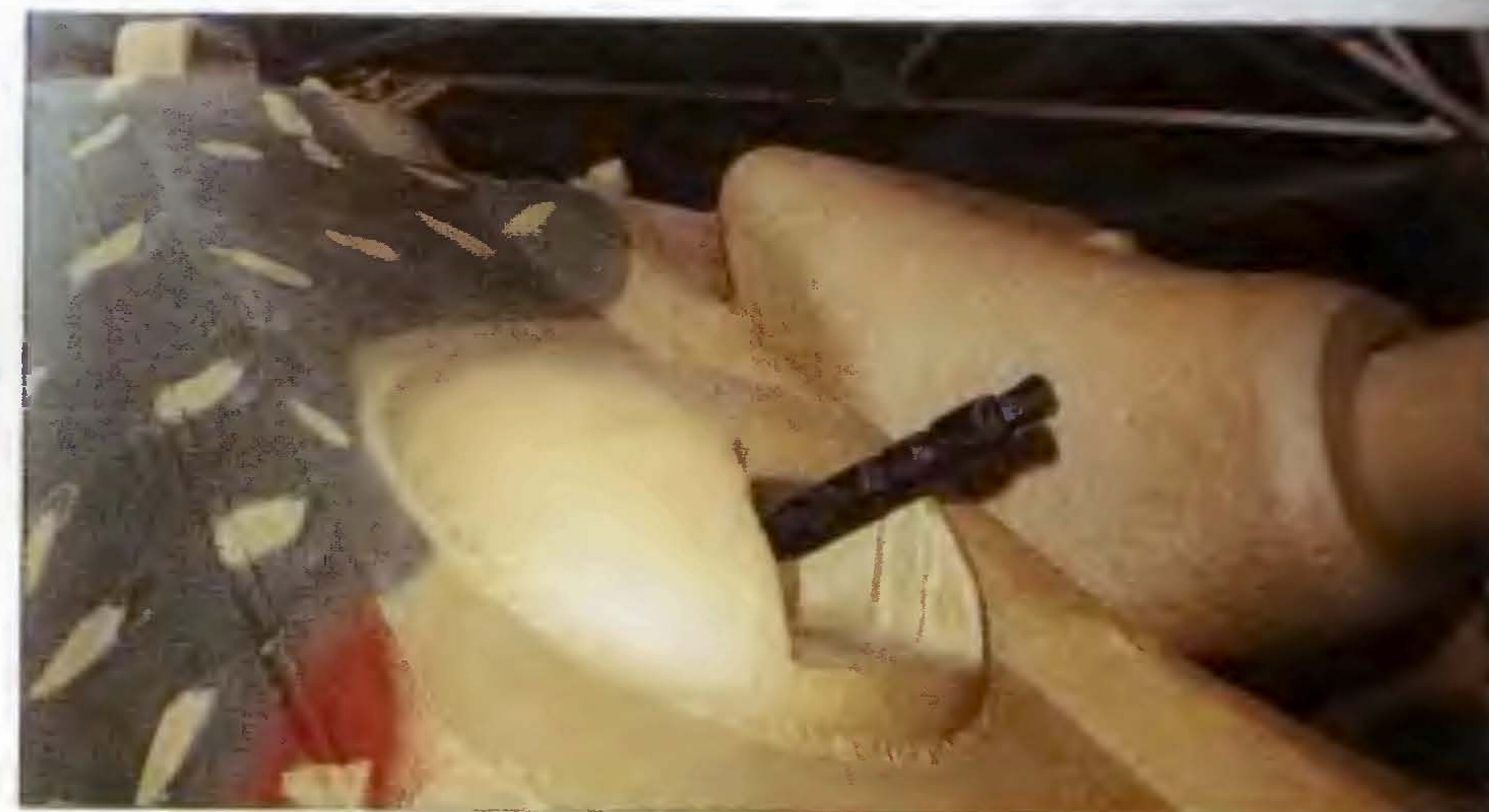
A bolted gun mount collar and a late mantlet of "Jagdpanther" Tank Museum Bovington. Note 8.8 cm Pak 43/3 gun and monocular driver's periscope without rain shield. [JN]
