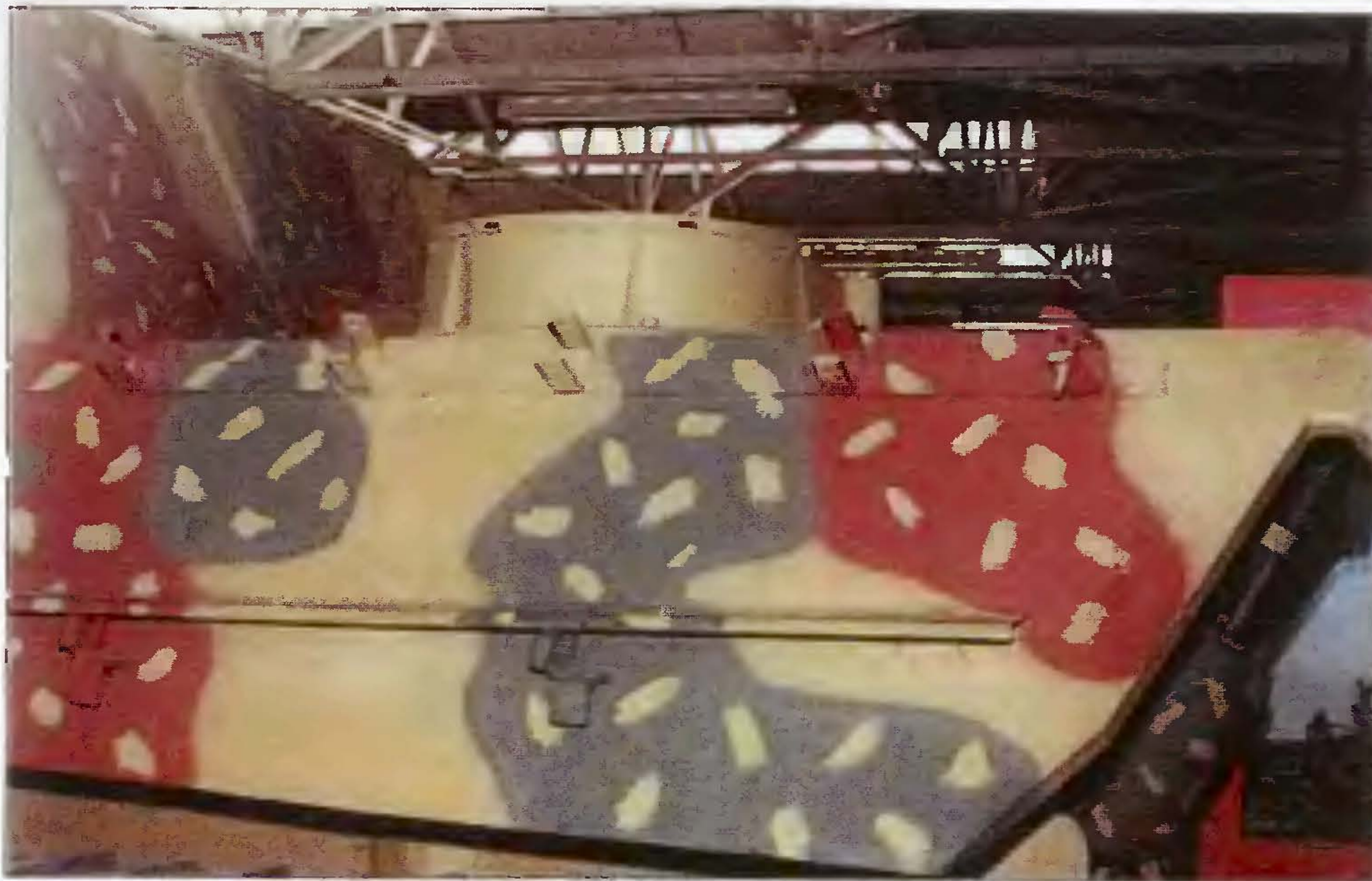
Hull side with spare track links bracket, note the retaining pin with chain. Below side skirt (schürzem) support on the hull side. Note raised cover for the air intake fan. The high box protected an extra duct to engine section.
