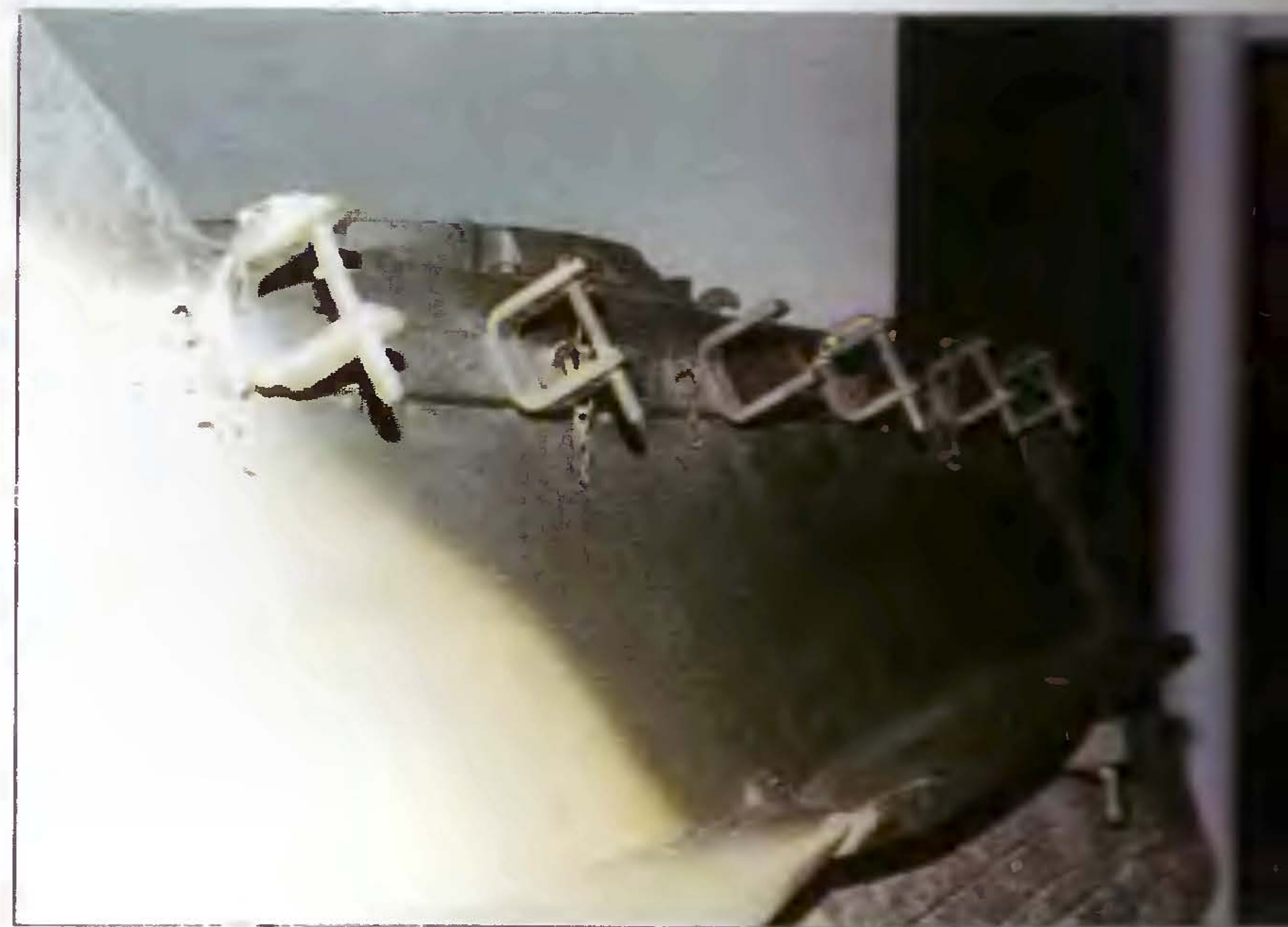
Hull side with spare track links bracket, note the retaining pin with chain. Note a damaged side skirt (schürzem) support.
