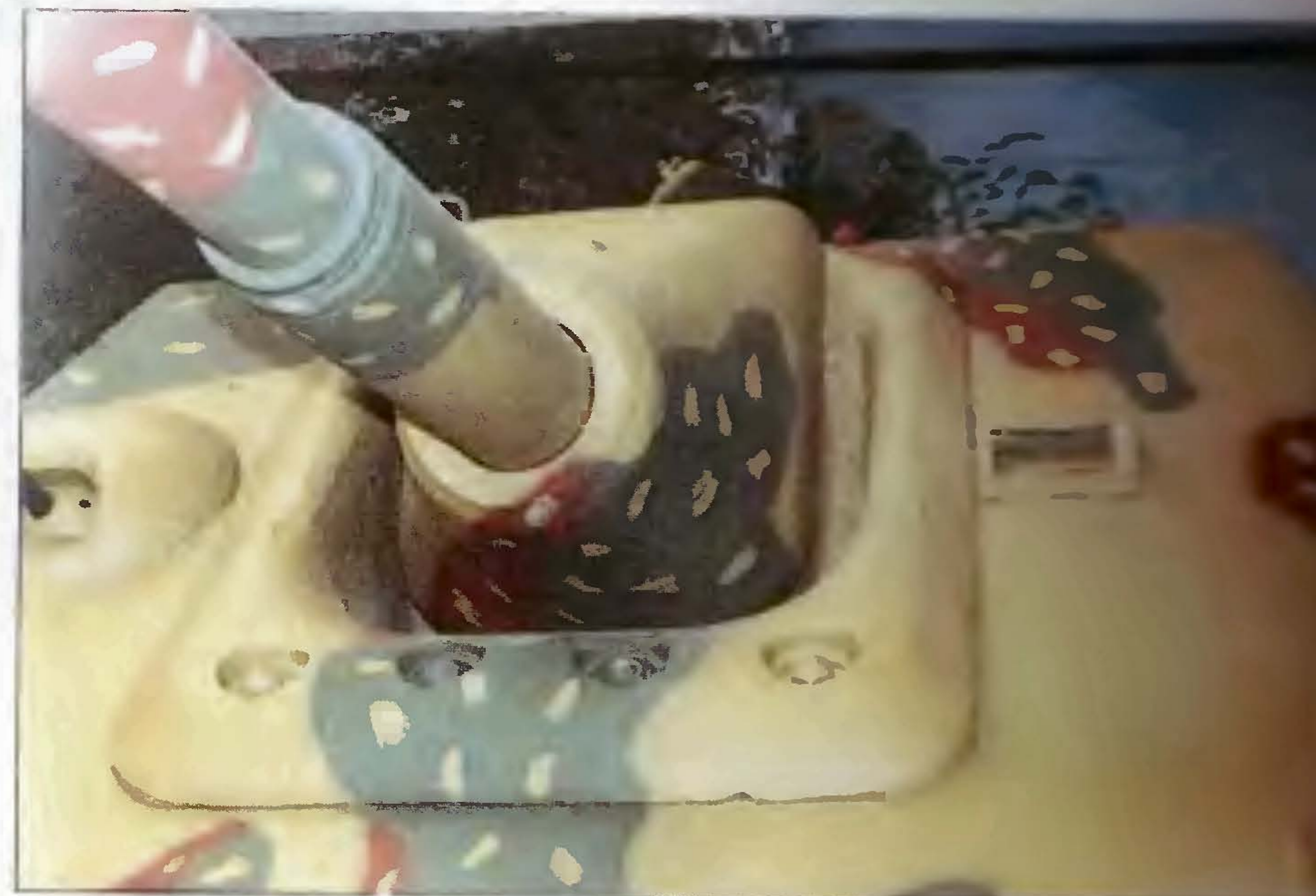
A bolted gun mount collar and a late mantlet of "Jagdpanther" Tank Museum Bovington. Note 8.8 cm Pak 43/3 gun and monocular driver's periscope without rain shield. [JN]
