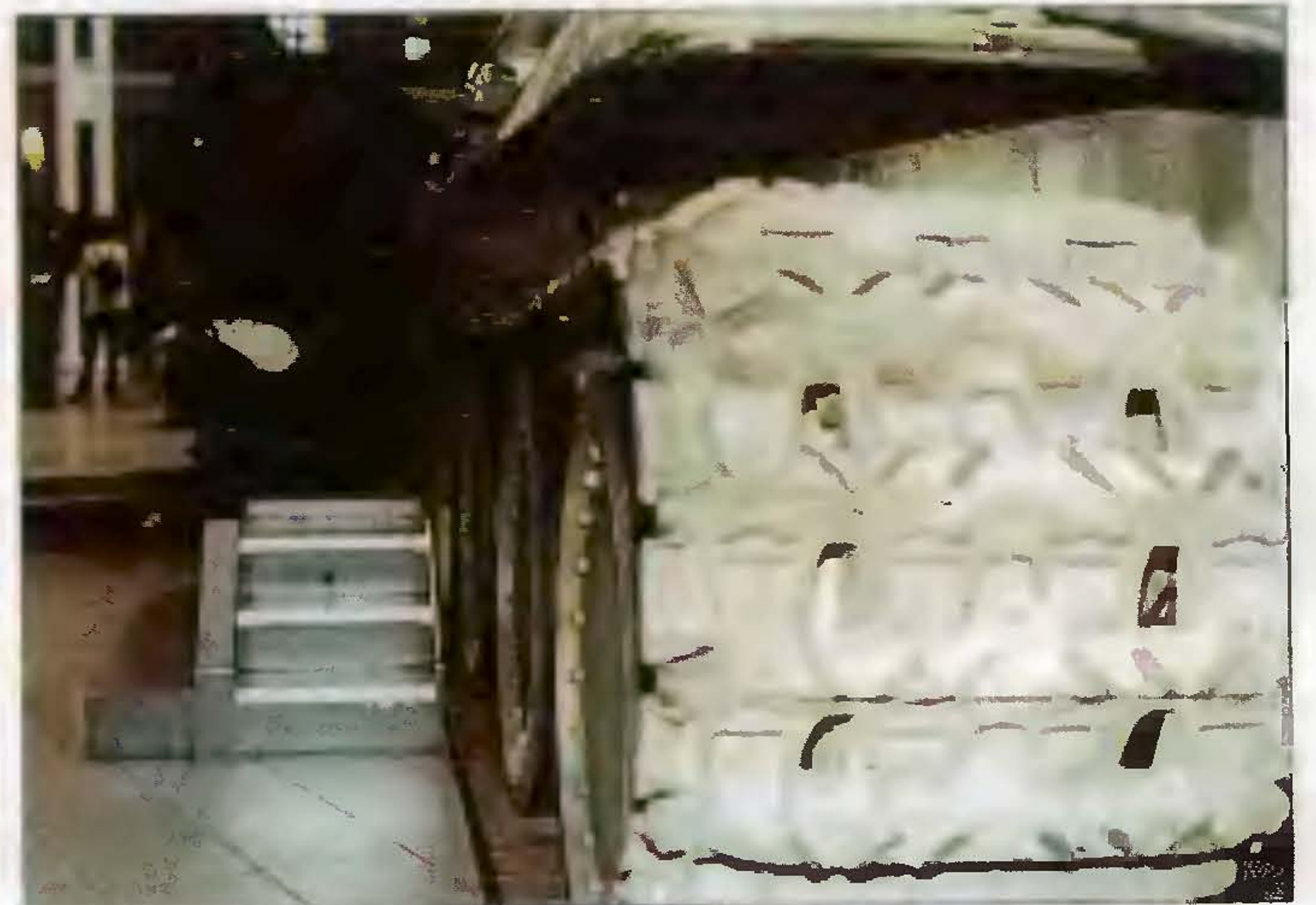
Below. Road wheels and Kgs 64/660/160 track links.
